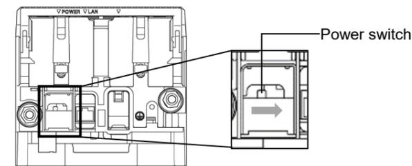
Initialization will take place after the power is turned on. This will take approximately 25 seconds. The process performs system checks and disables alarms, and performs other startup settings, then enters detection mode.
