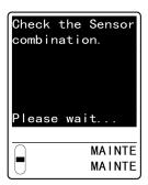
13 Press the TEST/ SET key when the screen indicates sensor replacement is complete.
