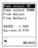
3 Press the ▲ key or ▼ key to select [Flow Adjust], then press the TEST/SET key.
