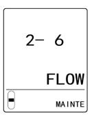
2 Press the ▲ key or ▼ key to increase or decrease the pump output so that the flow for [LineA] and [LineB] are each more than 0.28 L/min.
