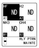
5 Press the ▲ key or ▼ key to select [ND] or [NE], then press the TEST/SET key.
