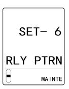
3 Press the ▲ key or ▼ key to select [FLT RLY], then press the TEST/SET key.
