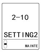
2 Press the ▲ key or ▼ key to select [SET- 4 TEST RLY], then press the TEST/SET key.
