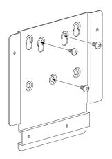
Mounting plate for three or four mounting screws
