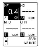
9 To record the results of span adjustment, press the TEST/SET key. Press the MODE key to skip recording.
