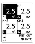
5 Press the ▲ key or ▼ key to select [2.5], [4-20], [HOLD], or [4.0], then press the TEST/SET key.
