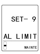
3 Press the ▲ key or ▼ key to select [ON] or [OFF], then press the TEST/SET key.
