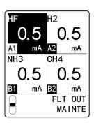
5 Press the ▲ key or ▼ key to select [0.5], [21.5], or [OPT], then press the TEST/SET key.
