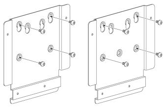
Mounting plate for four mounting screws
