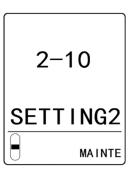
2 Press the ▲ key or ▼ key to select [SET- 5 TEST4-20], then press the TEST/SET key.
