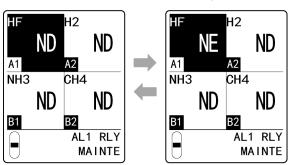
6 Press the ▲ key or ▼ key to select [ND] or [NE], then press the TEST/SET key.
