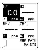
5 Introduce the gas for span adjustment, and press the TEST/SET key when the concentration stabilizes.
