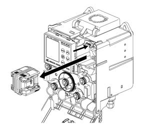
5 Match the new pump unit to the shape of the main unit and push into place.
