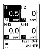
The second alarm is triggered when the concentration reaches the second alarm setpoint.
