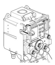
6 Grasp by the grips on the left and right of the fan unit and pull out.
