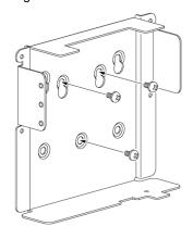
Mounting plate for three or four mounting screws
