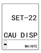
3 Press the ▲ key or ▼ key to select the fault code, then press the TEST/SET key.
