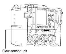
7 Grasp the projections on the left and right of the flow sensor unit and pull out.
