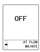
2 Press the ▲ key or ▼ key to select [SET- 3 MAINTE], then press the TEST/SET key.
