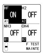
7 Press the ▲ key or ▼ key to select [OFF], then press the TEST/SET key.
