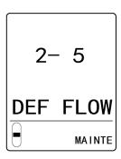
2 Press the ▲ key or ▼ key to select [Pump output UP] or [Pump output DOWN], then press the TEST/SET key. Select [Pump output UP] to increase pump output. Select [Pump output DOWN] to decrease pump output. Increase or decrease the output of the pump and adjust so that the connected flowmeter indicates 0.6 L/min ± 10 %.
