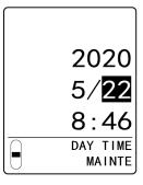
7 Press the ▲ key or ▼ key to set the hour (24-hour clock display), then press the TEST/SET key.
