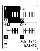
5 Press the ▲ key or ▼ key to select [H-HH], [L-LL], or [L-H], then press the TEST/SET key.
