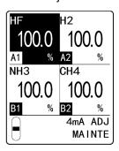
6 Press the ▲ key or ▼ key to adjust the output (%). Confirm that the ammeter reading is 20 mA and press the TEST/SET key.
