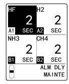
5 Press the ▲ key or ▼ key to set the alarm delay time, then press the TEST/SET key.
