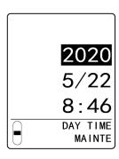
5 Press the ▲ key or ▼ key to set the month, then press the TEST/SET key.
