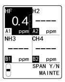
Span adjustment ends and the display returns to the display in step 2.
