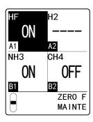
5 Press the ▲ key or ▼ key to select [ON] or [OFF], then press the TEST/SET key.
