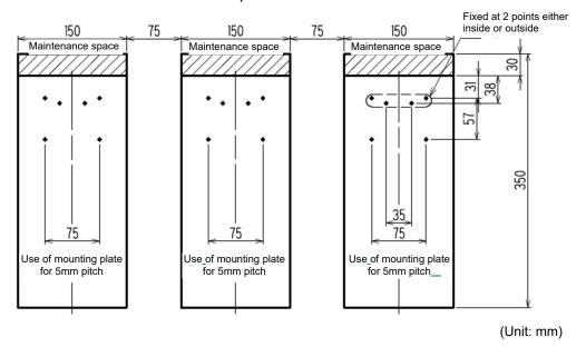
• When GD-70D is installed at a pitch of 10 mm
