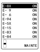
4 Press the ▲ key or ▼ key to select [ON] or [OFF], then press the TEST/SET key.
