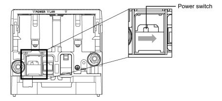
Initialization will take place after the power is turned on. This will take approximately 25 seconds. The process performs system checks and disables alarms, and performs other startup settings, then enters detection mode.
