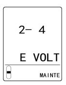
2 Check the set potential or element voltage.
