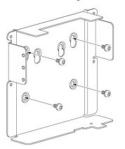
Mounting plate for four mounting screws
