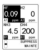
5 Press the ▲ key or ▼ key to select the zero suppression value, then press the TEST/SET key.
