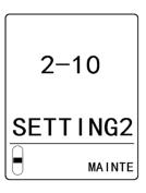
2 Press the ▲ key or ▼ key to select [SET- 2 SUPPRESS], then press the TEST/SET key.
