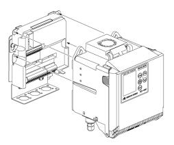
4 Pull the projection on the top of the main unit towards you to open the front cover.
