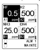
6 Press the ▲ key or ▼ key to set the alarm value for the second alarm setpoint, then press the TEST/SET key.
