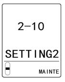
2 Press the ▲ key or ▼ key to select [SET-20 FLT RLY], then press the TEST/SET key.
