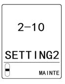
2 Press the ▲ key or ▼ key to select [SET- 1 DAY TIME], then press the TEST/SET key.
