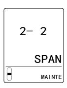
2 Press the ▲ key or ▼ key to select the sensor for which span adjustment is to be performed.
