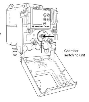
3 Pull the chamber switching unit towards you and turn to the left or right to place the nipple in the [CAL A] or [CAL B] position.
