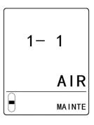
2 Press the ▲ key or ▼ key to select the sensor to be air calibrated.
