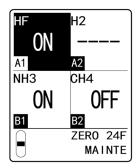
5 Press the ▲ key or ▼ key to select [ON] or [OFF], then press the TEST/SET key.
