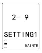
2 Press the ▲ key or ▼ key to select [SET- 2 ALM DLY], then press the TEST/SET key.
