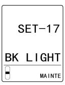
3 Press the ▲ key or ▼ key to select [ON] or [SAVE], then press the TEST/SET key.
