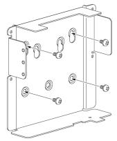
Mounting plate for three or four mounting screws
