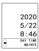
4 Press the ▲ key or ▼ key to set the last two digits of the year, then press the TEST/SET key.
