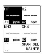
4 Press the TEST/SET key to confirm the sensor to be calibrated.
