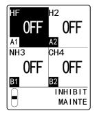
5 Press the ▲ key or ▼ key to select [OFF] or [ON], then press the TEST/SET key.
