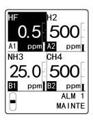
5 Press the ▲ key or ▼ key to set the alarm value for the first alarm setpoint, then press the TEST/SET key.
