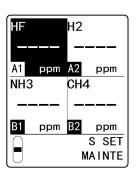
4 Press the TEST/SET key to enable the setting for the initial date of sensor use.
