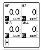
2 Press the ▲ key or ▼ key to select the sensor for which the alarm test is to be performed.
