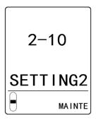
2 Press the ▲ key or ▼ key to select [SET-21 FLT OUT], then press the TEST/SET key.
