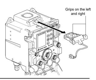
7 Match the fan unit to the shape of the main unit and push into place.
