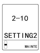
2 Press the ▲ key or ▼ key to select [SET-12 ZERO F], then press the TEST/SET key.
