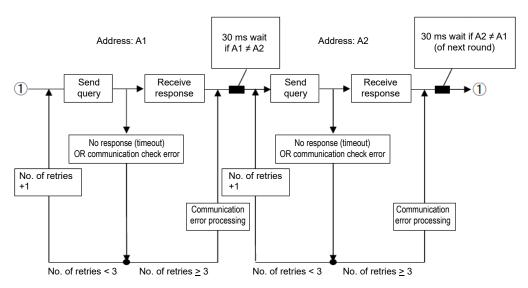
Example control station (e.g., PLC) communication procedure
