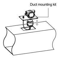
3 Insert the duct mounting kit into the opening in the duct. Secure in place with six M6 bolts.
