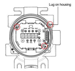
3 Pull out the display unit and hang on the lug on the housing.
