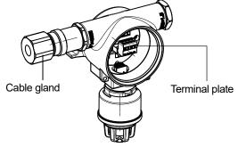
4 Pull out the terminal plate (TN1) from the terminal plate board.
