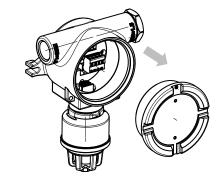
3 Attach a cable gland or conduit to the connector on the remote sensor head (GD-3).
