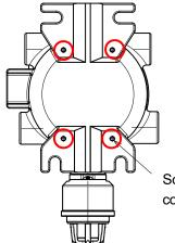
Screw holes on rear of container (four locations)
