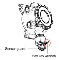
3 Rotate and remove the sensor guard.
