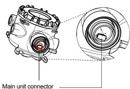
6 Confirm that the sensor is fully inserted.
