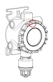
Take care not to trap the cable when attaching the cover. Rotate the cover clockwise until it moves no further to securely fasten in place.
