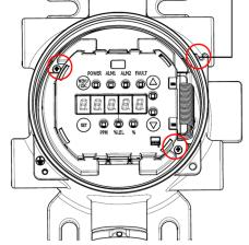
3 Pull out the display unit and hang on the lug on the housing.
