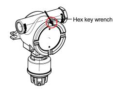
2 Rotate the cover counterclockwise and remove.
