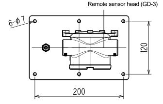
1 Cut out an opening in the top of the duct. Refer to the diagram to the right for the dimensions of the opening.
