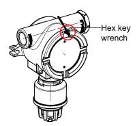
2 Rotate the cover counterclockwise and remove.
