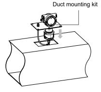
3 Insert the duct mounting kit into the opening in the duct. Secure in place with six M6 bolts.
