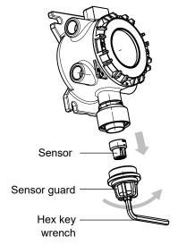
5 Match the main unit connector and sensor connector and fully insert the sensor.
