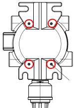
Bolt hole in the rear of the container (4 locations)
