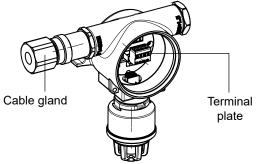
4 Pull out the terminal plate (TN1) from the terminal plate board.
