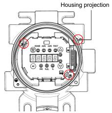
3 Take out the display unit and hook onto the housing projection.
