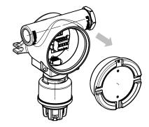
3 Attach a cable gland or conduit to the connector on the remote sensor head (GD-3).
