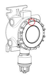
2 Unscrew the two M3 screws securing the display unit.
