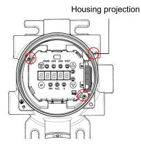
3 Take out the display unit and hook onto the housing projection.
