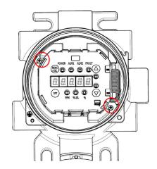
11 Rotate the cover clockwise to attach, and secure with the single M4 hex socket set screw.
