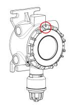
2 Unscrew the two M3 screws securing the display unit.
