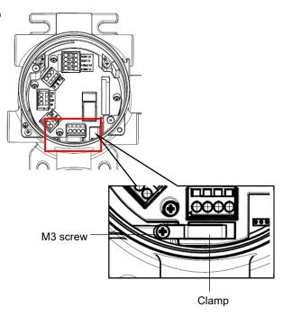
7 Connect the power and signal cables leading from the remote sensor head (GD-3) to the remote connection terminal plate.
