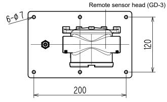
1 Cut the top panel of the duct to form a hole. Refer to the diagram at right for the dimensions of the hole.
