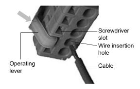
3 While continuing to press the operating lever, insert the cable into the wire insertion hole (round hole) until it touches the end.
