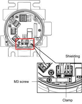
10 Return the display unit to its original position and secure with the two M3 screws.
