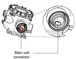
6 Confirm that the sensor is fully inserted.
