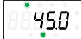
**6 Press the ▲ or ▼ key to adjust the reading to match the concentration of the gas introduced, then press the SET key.**
