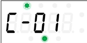
If the sensor mounted after replacement has the same or an older manufacturing date than the sensor replaced, the display alternates between [C-01] and [USEd], as follows.
