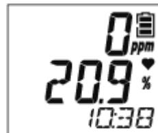
The buzzer blips twice, and the product switches to measurement mode.
