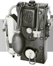
Riken type 18 gas detector (developed in 1952)
