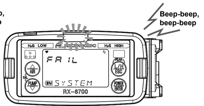
There are following alarm types: low flow rate, battery voltage abnormalities, calibration failure, sensor abnormalities, system abnormalities and clock abnormalities.
