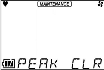
The LCD screen shows a heart icon in the top left, a 'MAINTENANCE' label in the top right, and a four-dot icon in the top right corner. At the bottom, the text 'PEAK CLR' is displayed in a large, blocky font.  | Press the <b>ENTER</b> button to goto the selection screen (P.53) |
