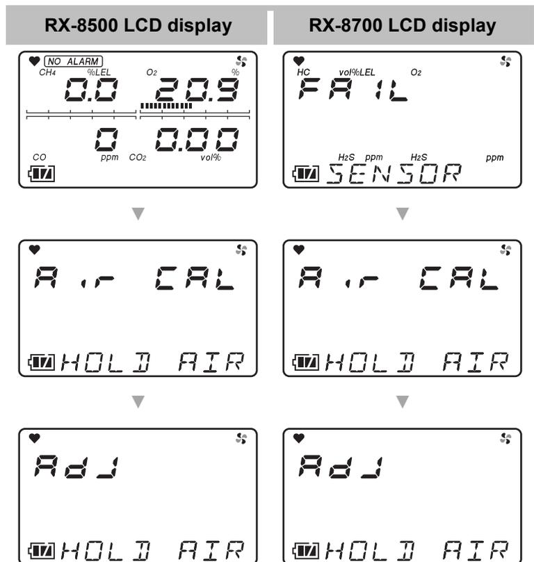
Keep the AIR button pressed while the screen shown in the right figure is displayed.
