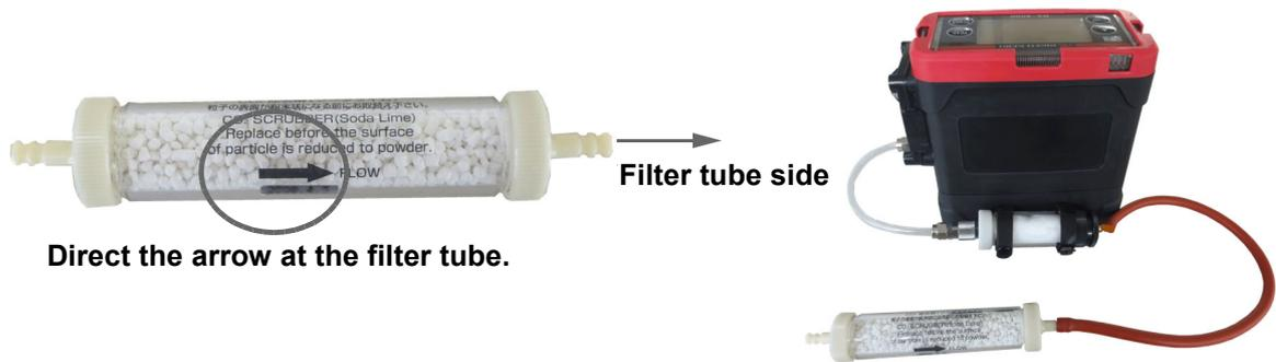
Stand the CO2 removal filter to use. With it laid horizontally, CO2 in the air may not be absorbed.
