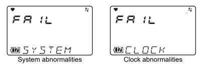
If a fault alarm is triggered, determine the cause and take appropriate action.
