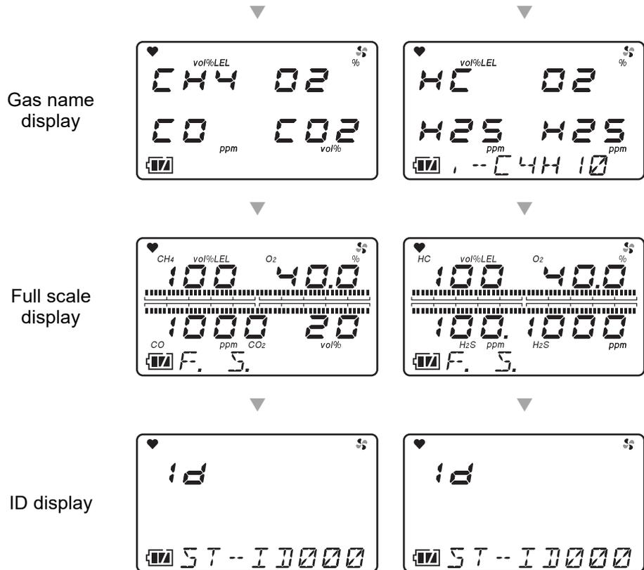
The screens on the right are displayed alternately until the **ENTER** button is pressed.
