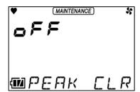
2 Press the **A** and **A** button to select ON or OFF, then press the **ENTER** button.
