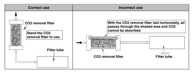
The number of usable times per filter depends on the carbon dioxide concentration in the air. It varies also by the air tightness of CO2 removal filter, storage temperature or humidity.
