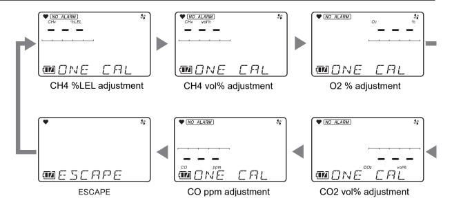
8. Maintenace 8-2. Span adjustment
