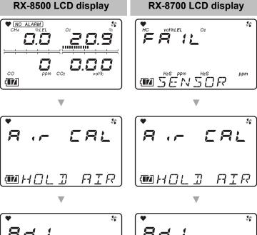
Keep the AIR button pressed while the screen shown in the right figure is displayed.
