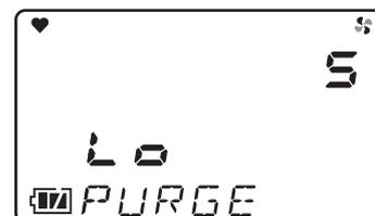
A purge operation is performed in the H<sub>2</sub>S [high concentration] measuring mode (HI) and then the HC/O<sub>2</sub>/H<sub>2</sub>S [low concentration] measuring mode (LO).
