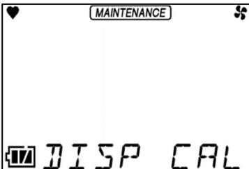
The LCD screen shows a heart icon in the top left, a 'MAINTENANCE' label in the top right, and a four-dot icon in the top right corner. At the bottom, the text 'DISP CAL' is displayed in a large, blocky font. | Press the <b>ENTER</b> button to goto the selection screen (P.53) |
