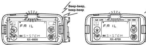
There are following alarm types: low flow rate, battery voltage abnormalities, calibration failure, sensor abnormalities, system abnormalities and clock abnormalities.
