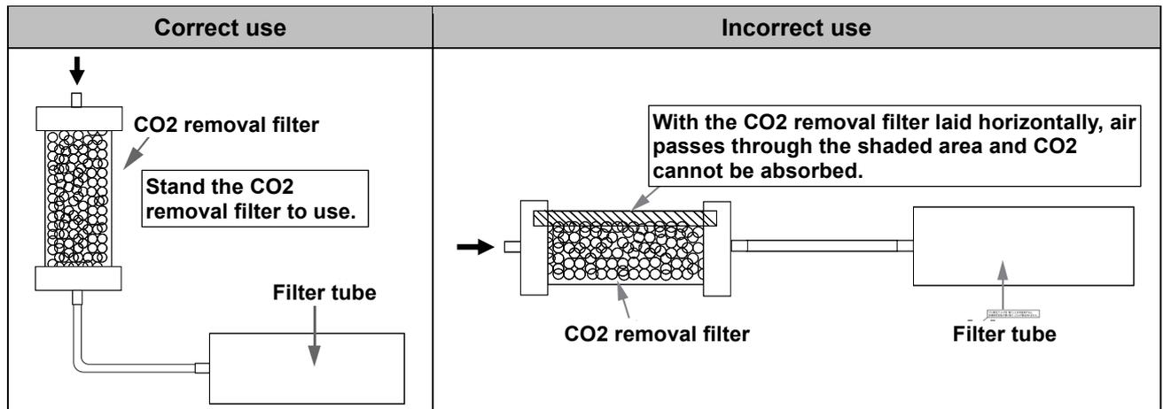
The number of usable times per filter depends on the carbon dioxide concentration in the air. It varies also by the air tightness of CO2 removal filter, storage temperature or humidity.
