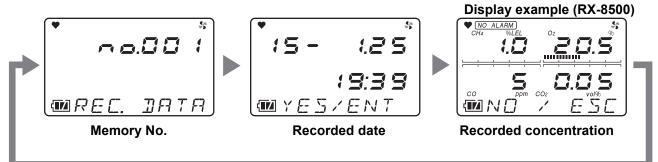
Press the ESC button to skip recording the displayed contents. The measurement screen returns.
