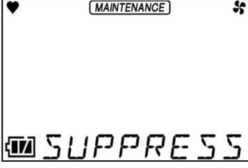
The LCD screen shows a heart icon in the top left, a 'MAINTENANCE' label in the top right, and a four-dot icon in the top right corner. At the bottom, the text 'SUPPRESS' is displayed in a large, blocky font.   | Press the <b>ENTER</b> button to goto the selection screen (P.52) |
