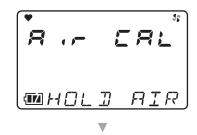
Keep the AIR switch pressed while the screen shown in the right figure is displayed.
