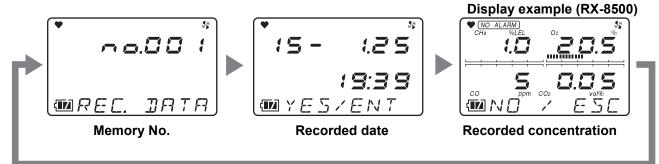
Press the ESC switch to skip recording the displayed contents. The measurement screen returns.
