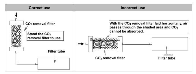
The number of usable times per filter depends on the carbon dioxide concentration in the air. It varies also by the air tightness of CO<sub>2</sub> removal filter, storage temperature or humidity.
