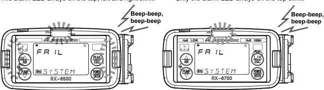
There are following alarm types: low flow rate, battery voltage abnormalities, calibration failure, sensor abnormalities, system abnormalities and clock abnormalities.
