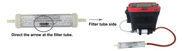
Stand the CO<sub>2</sub> removal filter to use. With it laid horizontally, CO<sub>2</sub> in the air may not be absorbed.
