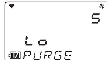
A purge operation is performed in the H<sub>2</sub>S [high concentration] measuring mode (HI) and then the HC/O<sub>2</sub>/H<sub>2</sub>S [low concentration] measuring mode (LO).
