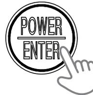
Hold down the switch until the entire LCD display and alarm lamp light up and the buzzer blips.
