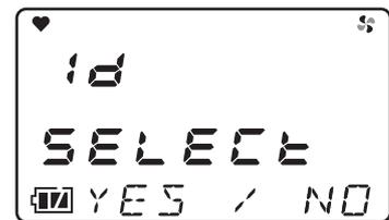
**2 Press the ENTER switch.****3 Select station ID with the ▲/▼ switch.**
