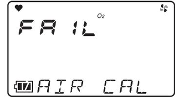
Air calibration failure display example
