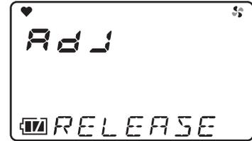
**3 For RX-8500, attach the CO<sub>2</sub> removal filter and press the ENTER switch.**
