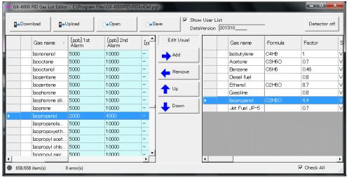
\* The calibration gas "Isobutylene" is automatically registered on the gas list and cannot be deleted.
