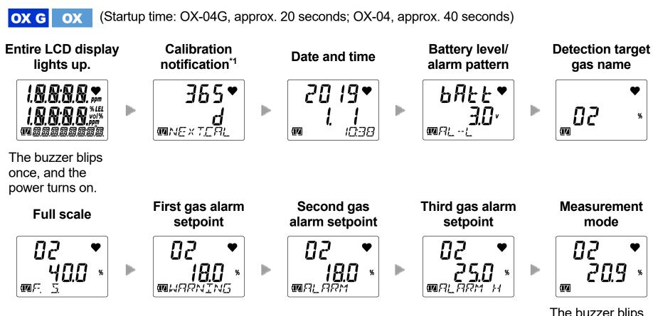
The buzzer blips twice, and the product switches to measurement mode.<sup>\* 2</sup>
