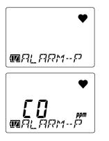
3 Press the POWER/MODE button several times to select the alarm type.
