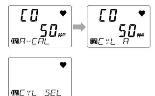
5 Press the AIR button several times to select the detection target gas, then press the POWER/MODE button.
