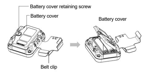
3 Remove the old batteries, then insert new batteries. Note the polarity.
