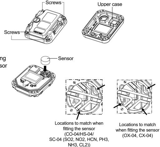
6 Return the upper case to its original position. Tighten the four screws with the Phillips head screwdriver.
