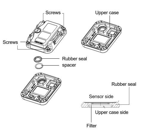
8 Return the upper case to its original position. Tighten the four screws with the Phillips head screwdriver.
