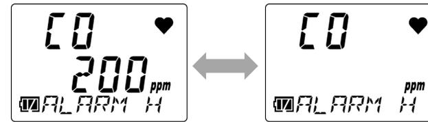
Display example: Carbon monoxide (CO) concentration: 200 ppm when the third alarm is triggered
