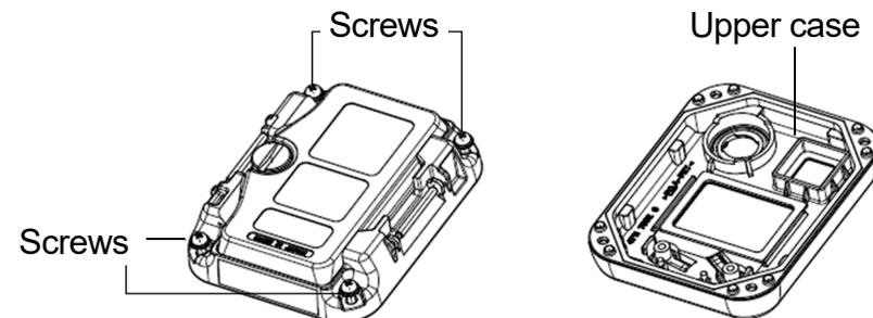
**5 Remove the filter, rubber seal, and dust filter from the upper case.**
