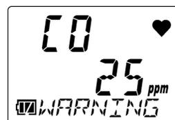
Furthermore, set as follows: First alarm  $\leq$  second alarm  $\leq$  third alarm (first alarm  $\geq$  second alarm for oxygen [O<sub>2</sub>]).
