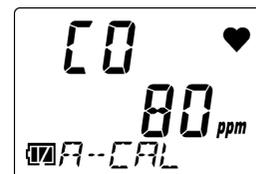
**4 Introduce the calibration gas, wait 60 seconds\*, then press the POWER/MODE button.**
