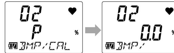
If the bump test fails [F] appears in the [BMP/CAL] screen (left side of middle row). Press the AIR button to view the reading at the time of the bump test.
