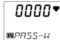
When you have set the 4th digit and press the POWER/MODE button, [END] appears. The display returns to the user mode menu.
