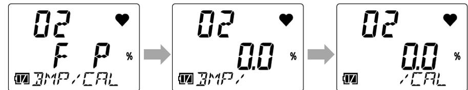
After a bump test failure, calibration is performed if specified in the setting. Once calibration is complete, the calibration result is displayed on the [BMP/CAL] screen (right side of middle row), then each time the AIR button is pressed, the display shows the reading at the time of the bump test and the calibration reading.
