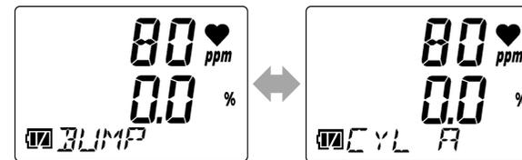
**3 Introduce the calibration gas, then press the POWER/MODE button.**
