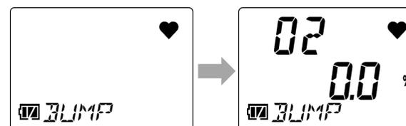
**2 Introduce the calibration gas, then press the POWER/MODE button.**
