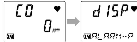
**2 Press the POWER/MODE button several times to select the alarm setpoint display [dISP ALARM-P].**
