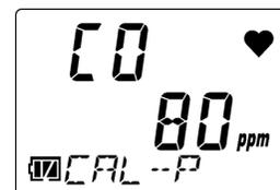
[END] appears once the settings are complete. The display returns to the [CAL-P] (target gas selection) screen.
