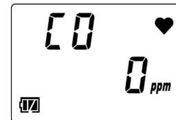
**2 Release the AIR button once the LCD display changes from [Air HOLD] to [AdJ RELEASE].**
