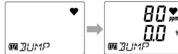
**2 Press the AIR button several times to select the cylinder for the bump test, then press the POWER/MODE button.**
