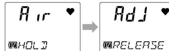
The product automatically returns to measurement mode once air calibration has been successfully completed.
