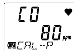
[END] appears once the settings are complete. The display returns to the [CAL-P] (target gas confirmation) screen.
