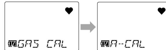
**2 Press the AIR button several times to select [A-CAL], then press the POWER/MODE button.**
