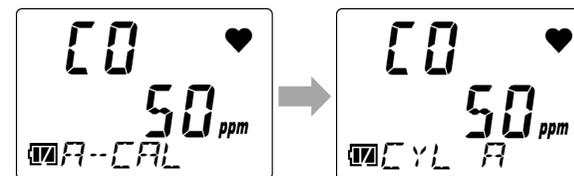
**4 Press the AIR button several times to select [CYL SEL], then press the POWER/MODE button.**
