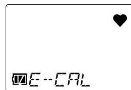
**2 Press the AIR button several times to set the time for quick calibration, then press the POWER/MODE button.**
