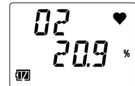
The buzzer blips twice, and the product switches to measurement mode.\*2
