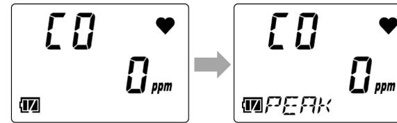
**2 Press the POWER/MODE button to cycle through the items displayed.**
