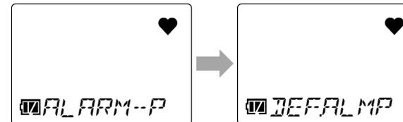
**2 Press the AIR button several times to select [DEF.ALMP], then press the POWER/MODE button.**
