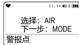
每次按下 AIR 按钮，按“全尺寸” → “WARNING” → “ALARM” → “ALARM H” → “STEL” → “TWA” → “全尺寸” → ··· 的顺序显示。
