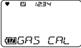
The LCD display shows a battery icon, a heart icon, a 'M' icon, and the number '1234' at the top. Below this, the words 'GAS CAL' are displayed in a large, pixelated font.    | P. 44                |
