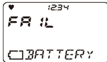
Battery voltage abnormality
