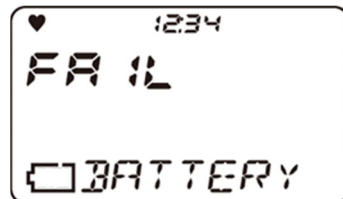
Battery voltage abnormality
