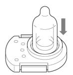
4 Place the pellet into which the lamp has been fitted on a flat surface. Place the VOC sensor main unit over it and press so that the pellet fits into the VOC sensor main unit.
