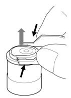
4 Place the pellet and lamp on a clean surface. Separate the pellet removal tool from the VOC sensor.
