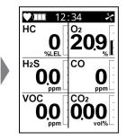
The buzzer blips twice and the normal measurement mode measurement screen is displayed.
