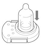
4 Place the pellet into which the lamp has been fitted on a flat surface. Place the VOC sensor main unit over it and press so that the pellet fits into the VOC sensor main unit.
