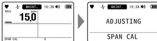
The following results are displayed when the bump test and gas adjustment end.
