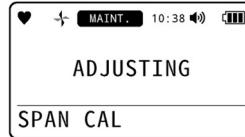
Once span adjustment has been successfully completed, the result is displayed, and the concentration after span adjustment is then displayed.
