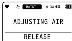
Once fresh air adjustment has been successfully completed, the result is displayed, and the concentration after fresh air adjustment is then displayed.
