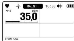
Span adjustment is performed.
