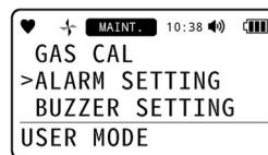
2 Press the **▲/AIR** or **RESET/▼** button to select **[ALARM TYPE]**, then press the **POWER/ENTER** button.
