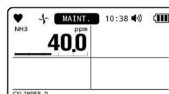
4 Introduce the calibration gas for span adjustment, wait 60 or 120 seconds, then press the POWER/ENTER button.
