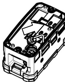
5 Remove the packing and dust filter from the filter section.
