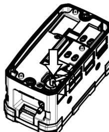
9 Tighten the two screws on the bottom of the main unit to secure the battery unit.
