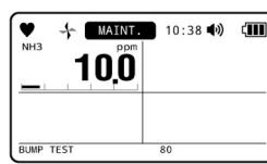
If the bump adjustment function is enabled, the product will automatically perform gas adjustment in the event of a bump test failure.
