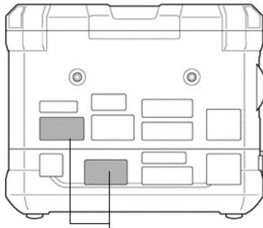
Typical nameplates for explosion-proof electrical equipment type certified (Japan EX) models
