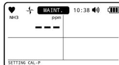
5 Press the ▲/AIR or RESET/▼ button to set the gas concentration for span adjustment, then press the POWER/ENTER button.
