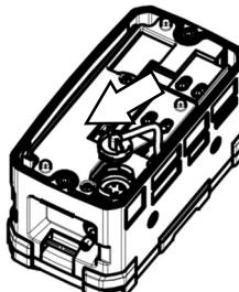
8 Turn the filter section clockwise to secure it.
