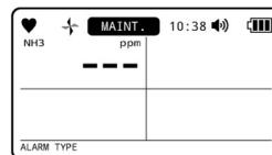
4 Press the **▲/AIR** or **RESET/▼** button to select an alarm type.
