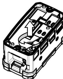
4 Remove the tube from the filter nipple.
