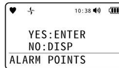
3 Press the ▲/AIR button several times to display the alarm setpoint for the alarm test.
