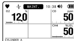
4 Introduce the calibration gas for span adjustment, wait 60 seconds, then press the POWER/ENTER button.
