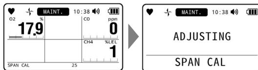
The following results are displayed when the bump test and gas adjustment have ended.
