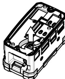
**4 Remove the tube from the filter nipple.**
