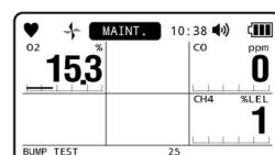
If the bump adjustment function is enabled, the product will automatically perform gas adjustment in the event of a bump test failure.
