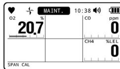
Span adjustment is performed.
