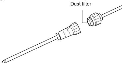
**3 Rotate the probe to attach it.****NOTE**
