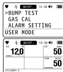
2 Press the ▲/AIR or RESET/▼ button to select the cylinder to be adjusted, then press the POWER/ENTER button.
