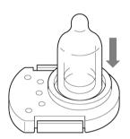
4 Place the pellet into which the LED has been fitted on a flat surface. Place the VOC sensor main unit over it and press so that the pellet fits into the VOC sensor main unit.
