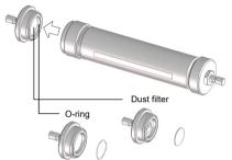
3 Turn the cap (M thread) to attach it to the filter tube with flow monitor.
