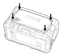
2 Remove the cover and take out the VOC sensor. Grasp the cylindrical part of the sensor and gently pull out.
