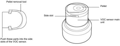
3 Press the pellet removal tool on both sides to lift the pellet and LED from the VOC sensor main unit.
