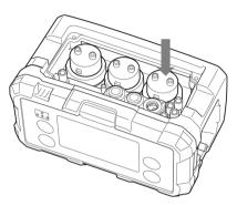
2 Use the four screws to secure the cover on the top of the main unit.
