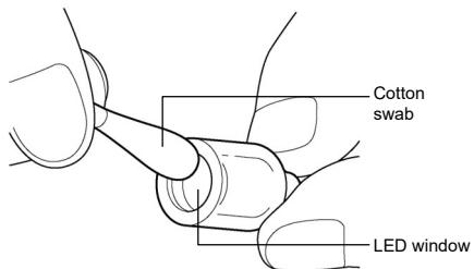
3 Use a clean cotton swab to remove any remaining alumina polishing powder from the LED window.
