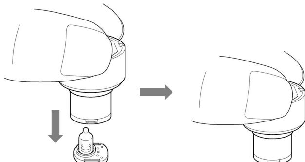
**<Installing the VOC sensor>**
