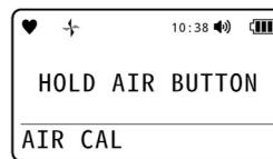
**2 Release the ▲/AIR button once [RELEASE] appears on the screen.**
