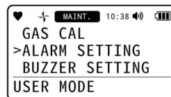
2 Check to confirm that **[ALARM POINTS]** is selected, then press the **POWER/ENTER** button.
