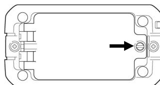
**2 Open the battery cover.****3 Insert six new AA alkaline batteries.**
