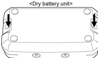
**2 Remove the battery unit.**
