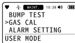
2 Press the ▲/AIR or RESET/▼ button in the [GAS CAL] menu to select [SPAN CAL], then press the POWER/ENTER button.
