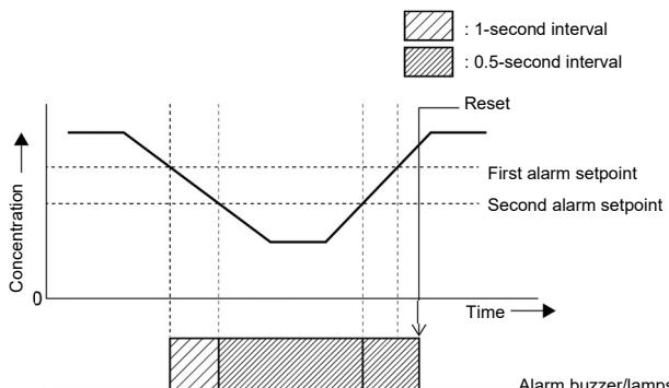
**<Alarm pattern (L-H) (oxygen deficiency alarm)>**
