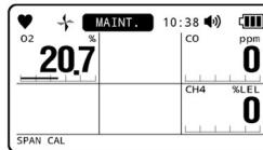
Span adjustment is performed.
