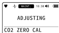
Once CO<sub>2</sub> zero adjustment has been successfully completed, the result is displayed, and the concentration after CO<sub>2</sub> zero adjustment is then displayed.
