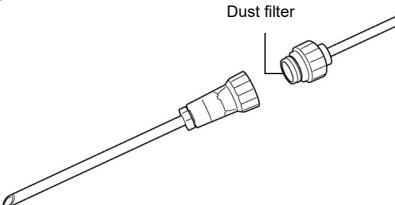
**3 Rotate the probe to attach it.****NOTE**
