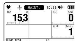
If the bump adjustment function is enabled, the product will automatically perform gas adjustment in the event of a bump test failure.
