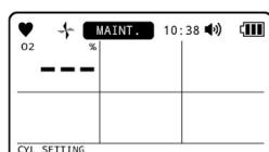
5 Press the **▲/AIR** or **RESET/▼** button to set the sensor, then press the **POWER/ENTER** button.
