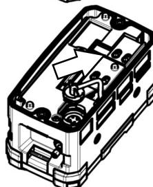
**5 Remove the packing and dust filter from the filter section.**
