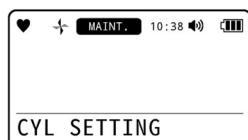
4 Press the **▲/AIR** or **RESET/▼** button to select the sensor, then press the **POWER/ENTER** button.
