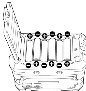
**4 Close the battery cover, then tighten the battery cover retaining screw.**
