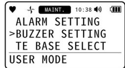
**2 Press the ▲/AIR or RESET/▼ button to select a buzzer setting.**
