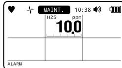
6 Press the ▲/AIR or RESET/▼ button to set the value for the STEL alarm setpoint, then press the POWER/ENTER button.
