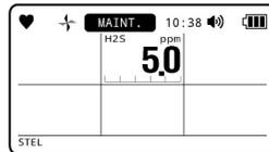
7 Press the ▲/AIR or RESET/▼ button to set the value for the TWA alarm setpoint, then press the POWER/ENTER button.
