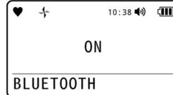
The Bluetooth device connection is set. [SETTING] appears followed by [END], and the display returns to the screen in Step 1.
