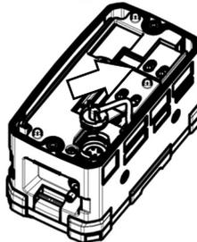
**5 Remove the packing and dust filter from the filter section.**
