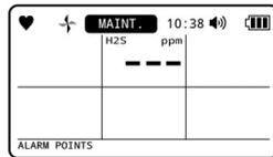
4 Press the ▲/AIR or RESET/▼ button to set the value for the first alarm setpoint, then press the POWER/ENTER button.
