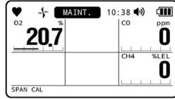
Span adjustment is performed.
