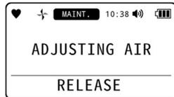
Once fresh air adjustment has been successfully completed, the result is displayed, and the concentration after fresh air adjustment is then displayed.
