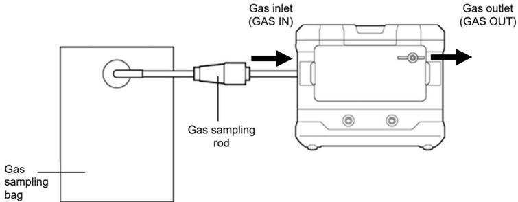
**<When using the CF-284 CO<sub>2</sub> removal filter>**
