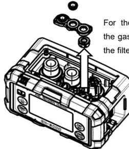
For the R sensor, remove the gasket and then remove the filter/sensor.
