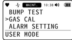
2 Press the ▲/AIR or RESET/▼ button in the [GAS CAL] menu to select [CO2 ZERO CAL], then press the POWER/ENTER button.
