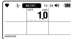
5 Press the ▲/AIR or RESET/▼ button to set the value for the second alarm setpoint, then press the POWER/ENTER button.
