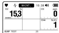
If the bump adjustment function is enabled, the product will automatically perform gas adjustment in the event of a bump test failure. The gas adjustment remaining time is displayed at the bottom of the screen.
