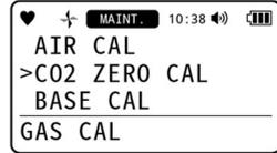
3 Introduce nitrogen (N<sub>2</sub>), wait 60 seconds, then press the POWER/ENTER button.
