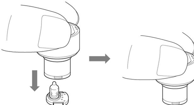
**<Installing the VOC sensor>**
