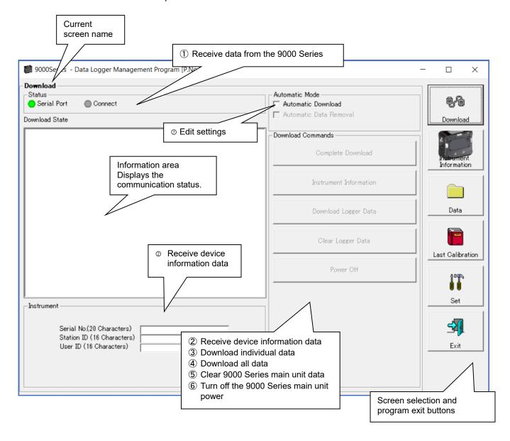
To start data communication, connect using a USB cable, start this program, and turn on the main unit. The program will automatically determine whether data communication is possible; if so, it will enter reception standby mode.
