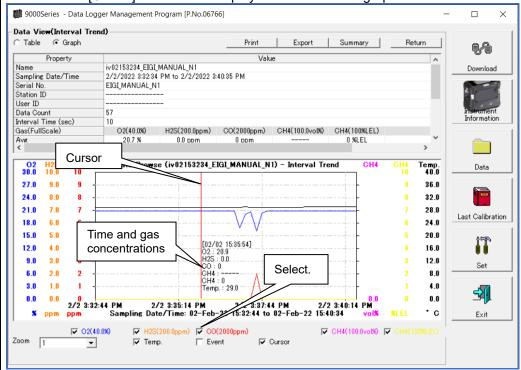
Use the  $\leftarrow$  and  $\rightarrow$  keys to move the cursor left and right. Use the  $\uparrow$  and  $\downarrow$  keys to move the time and concentration display up and down.
