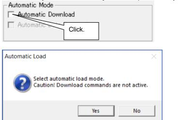
Click [Yes] to switch to automatic processing and to download data from the main unit automatically when communication is performed next.
