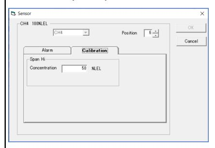
The [Span Lo] area is displayed only for sensors that allow double-range adjustment.
