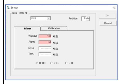
If the magnitude relationship between the warning and alarm setpoint values is inappropriate for the [LO]/[HI] or alarm type selection, the values are displayed with a pink background and the [OK] button is disabled.
