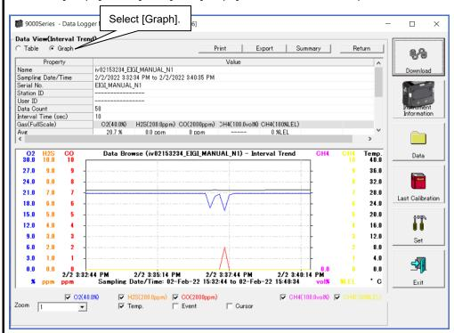
Various operations are available using the checkboxes and combo boxes at the bottom of the screen.
