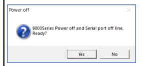
Click [Yes] to begin the process of turning off the 9000 Series main unit power and to reset the PC serial port before switching to standby to await data from the main unit.
