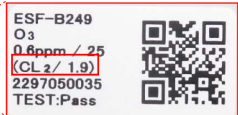
Typical label indicating replacement gas and conversion factor (Example: Replacement gas: Chlorine (Cl 2 ), conversion factor: 1.9)
