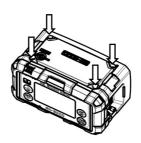
2 Remove the filter/sensor.
