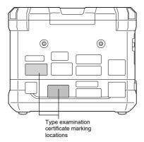
Typical nameplates for explosion-proof electrical equipment type certified (Japan EX) model
