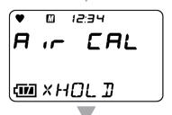
3 Release the AIR button once [RELEASE] is displayed. Fresh air adjustment is performed.
