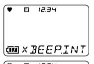
2 Press the AIR button to select the beep interval.
