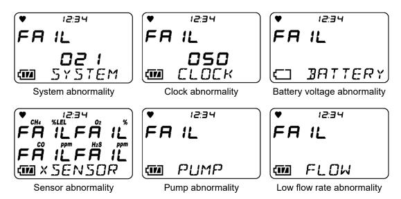
If a fault alarm occurs, determine the cause and take appropriate action.
