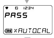
The concentration after AUTO adjustment is displayed. With Japan EX specifications, the concentration and sensor reserve value after AUTO adjustment are displayed after AUTO adjustment has been successfully performed.
