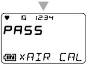
The current concentration appears after fresh air adjustment and the display returns to the screen in Step 1.
