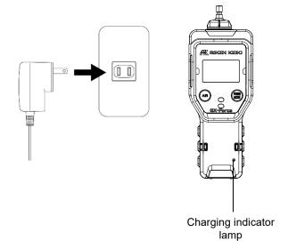
4 When charging is complete, unplug the charger from the outlet and close the USB protective cover.
