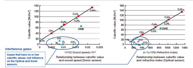
"Opt-Sonic calculation" using measuring results of the Optical sensor and Sonic sensor can minimize the interference effects caused by interference gases, and realize a high-accuracy measurement.
