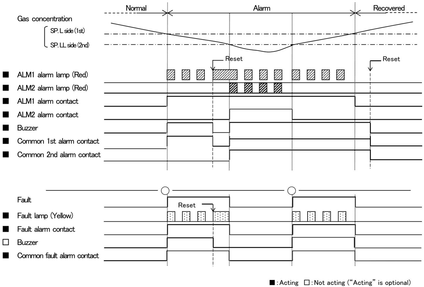
7. Gas alarm(L-H, self-latching)/Fault alarm(auto-reset)
