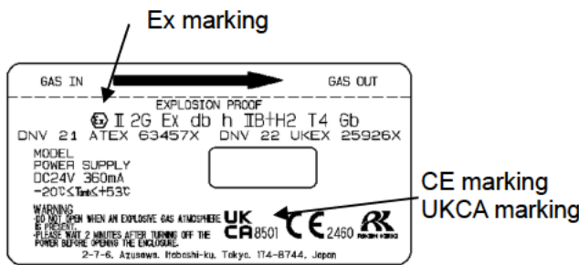
ATEX/ CE/UKCA marking type name plate (DC power specification only)
