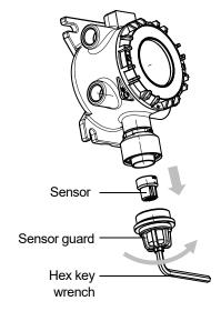
5 Match the main unit connector and sensor connector and fully insert the sensor.
