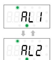
4 Press the ▲ or ▼ key to set the alarm setpoint, then press the SET key.
