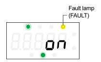
5 Once the fault test is complete, press the ▲ or ▼ key to select [oFF], then press the SET key.
