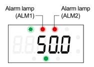
6 Once the alarm test is complete, press the MENU/ESC key. Returns to the [2-0.1] display.
