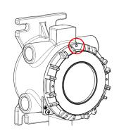
2 Unscrew the two M3 screws securing the display unit.
