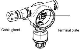
Pull out the terminal plate (TN1) from the terminal plate board.
