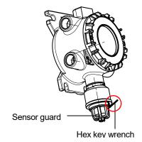
3 Rotate and remove the sensor guard.
