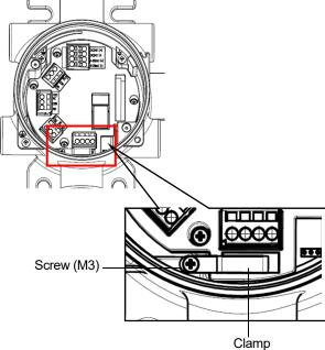
7 Connect the power and signal cables extending from the remote sensor head (GD-3) to the remote connection terminal plate.
