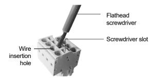
With the flathead screwdriver still being inserted, insert the cable into the wire insertion hole (round hole) until it contacts the end.
