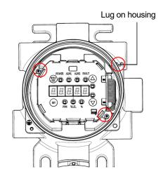
3 Pull out the display unit and hang on the lug on the housing.
