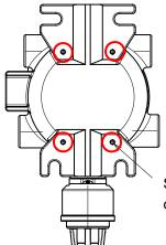
Screw holes on rear of container (four locations)
