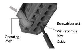
While continuing to press the operating lever, insert the cable into the wire insertion hole (round hole) until it contacts the end.
