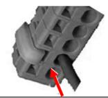
While holding down the lever, insert the wire into the (round) wiring hole until it reaches the deepest point. Once the lever is released, the wire is secured.
