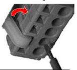
Push the lever with your finger to lower the spring in its inside.
