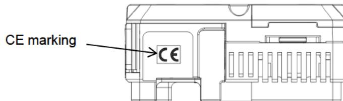
CE marking label (Bottom of instrument)
