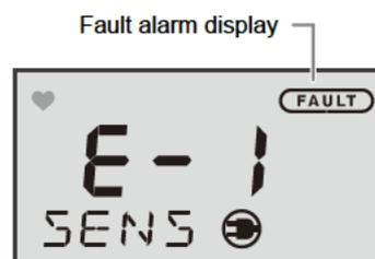
After the monitor is successfully returned from the fault, it restarts with the process normally performed right after it is turned on (initial clear).
