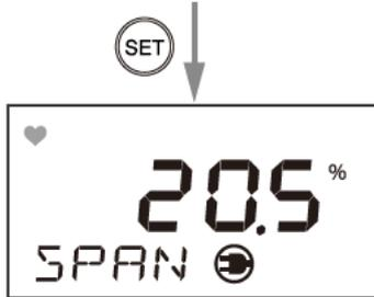
Press the concentration **SET** button again. While the concentration display is blinking, use the **↓** or **↑** button to adjust the reading to "20.9%".
