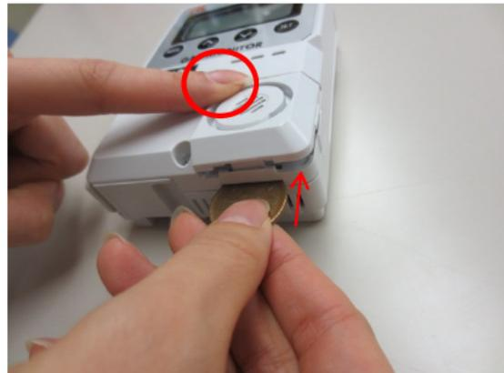
Remove the sensor cover to check the sensor.
