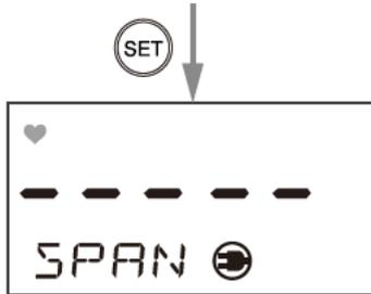
"PASS" is displayed when adjustment is completed, and "FAIL" is displayed when it fails.
