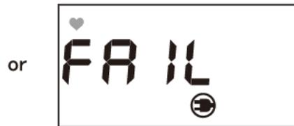
If "FAIL" is displayed, perform span adjustment again.
