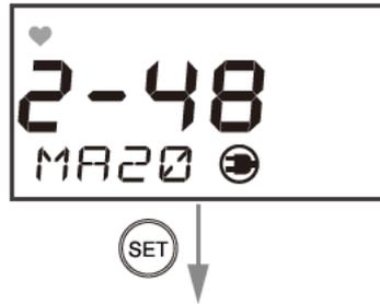
When "Adj" is displayed, connect an ammeter. Then, use the or button to adjust the value to 4 mA or 20 mA and press the **SET** button to confirm it.
